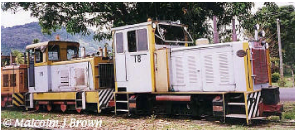
Fiji Oct/Nov 1994: Malcolm J Brown Collection from the CaneSIG website. #18 Hunslet 6wD, #15 Baguley-Drewry 0-6-0D
