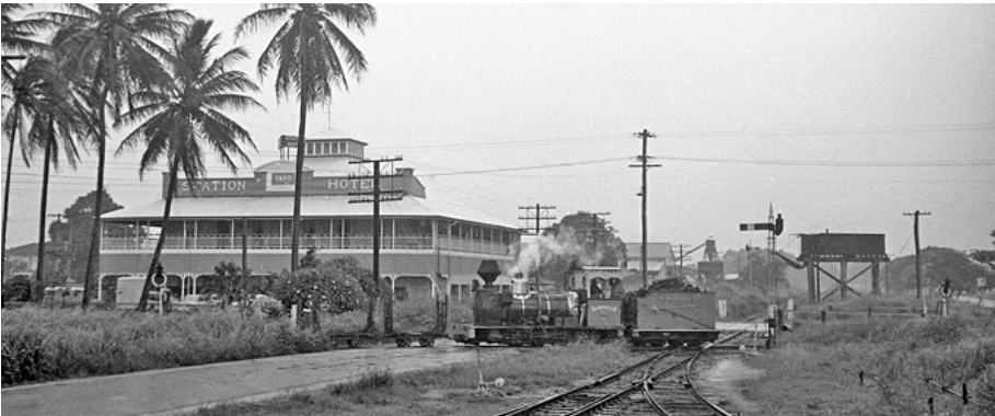
Victoria Mill Hudswell Clarke with a cane train crosses the QGR main line at Ingham station with the Station Hotel in the background, 1964. Peter Bruce photographer (when touring the north as a teenager).
