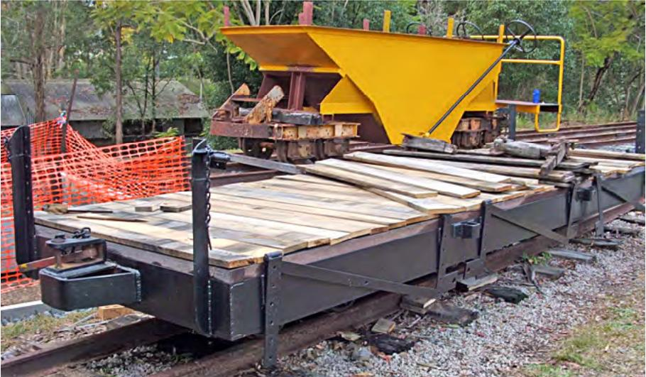
Progress to August 2011 showing floor boards loose and ready to fixed into position, with our rebuilt ballast wagon behind. Mark Gough photographer
