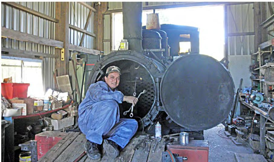
New member Brad Bell works on Bundy No 5, helping to dismantle the loco for new tubes and other work, 30 June 2012. Bob Gough photographer.
