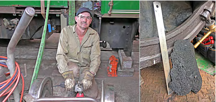
Ex-Dreamworld Perry work party, 9 October 2016. Mark Gough (left) cleaning the trailing axle in preparation for painting, Bob Gough photographer, and a large lump of carbon from the smoke stack (right), almost 200mm high by 25mm thick. Mark Gough photographer.
