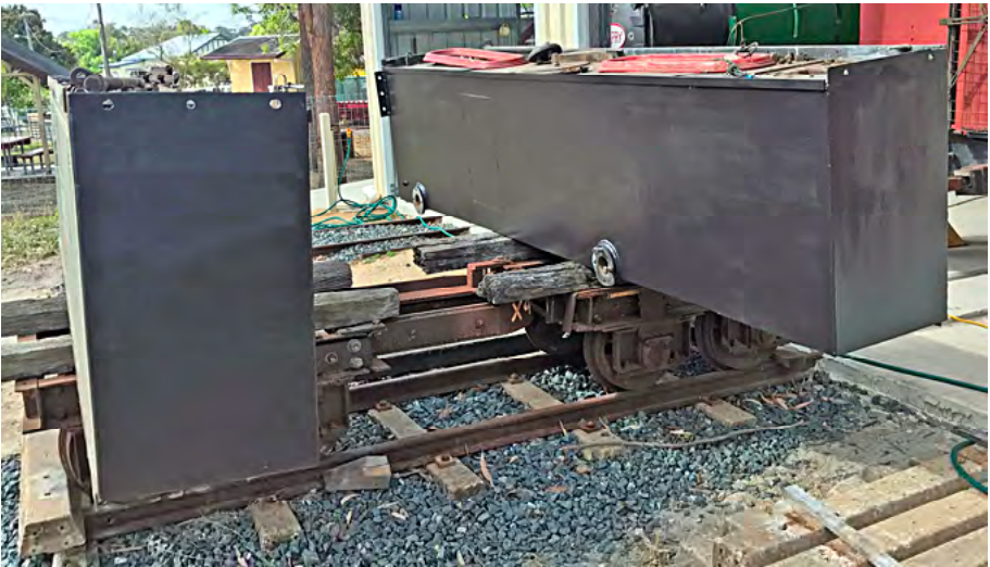
Perry side tanks being repainted by Sam Erb, 16 Sept 2018. Terry Olsson Photographer.
